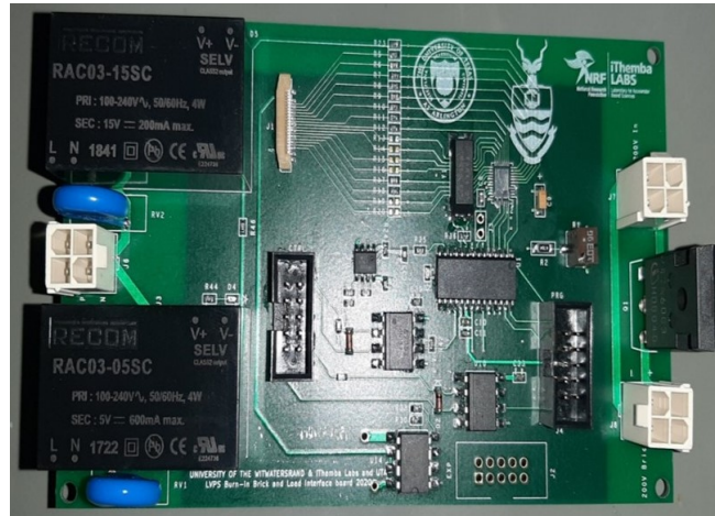
Figure 3: BI board prototype for burn-in station.
